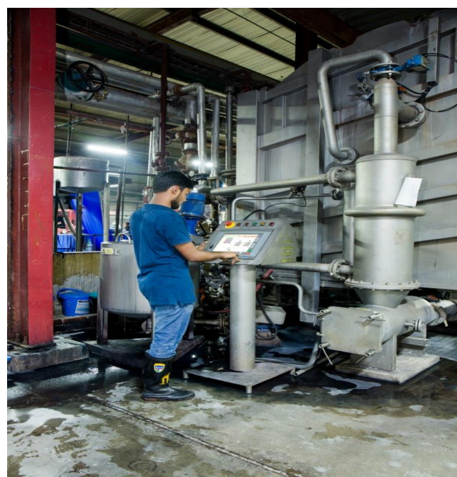
An operator running a Dyeing machine of cap 750kg used for gray fabrics dyeing
