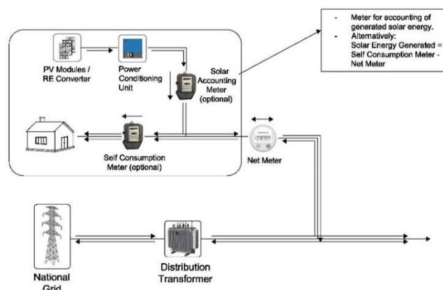
**Figure:** Typical Net Energy Metering Architecture.
