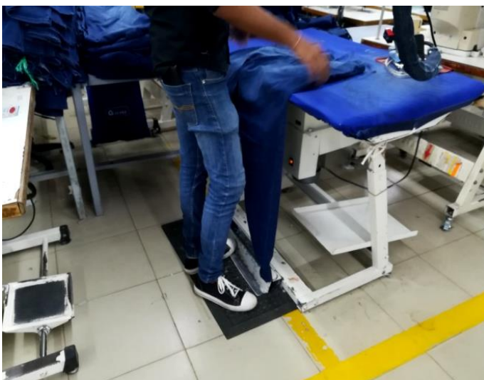
Carpet for workers where one worker is working in standing position
