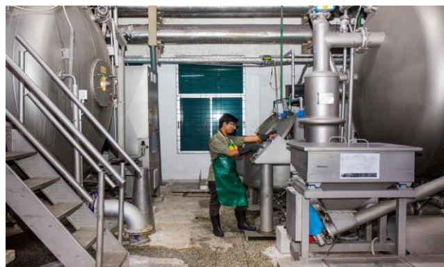
An operator using the Commanding Device of Sclavos ATHENA 3D used at Fabric Dyeing
