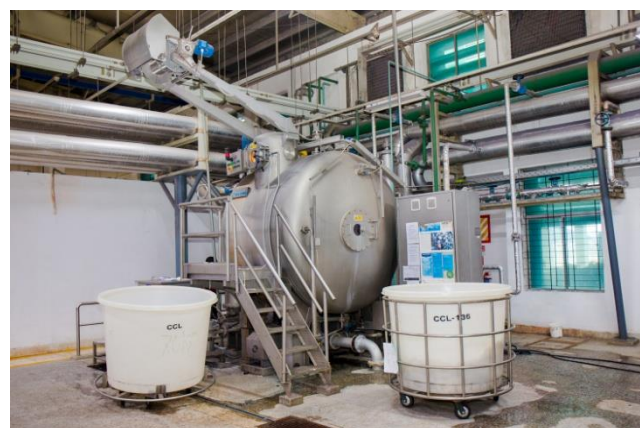
Sclavos ATHENA 3HT Fabric Dyeing Machine
