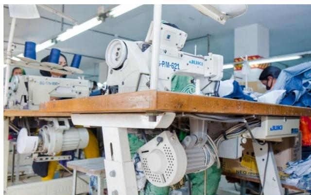
Servo Motor could be installed separately replacing the clutch motor
