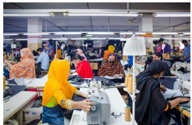
Workers using Sewing Machine equipped with Servo Motor at Bottom Gallery Pvt Ltd, Dhaka
