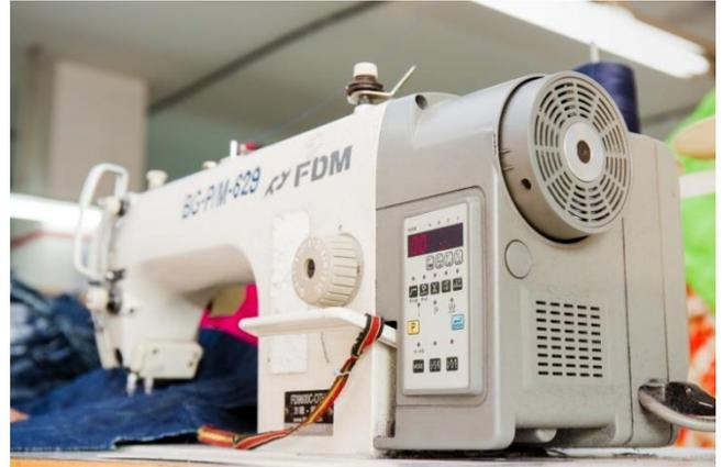
Sewing machine with Servo Motor
