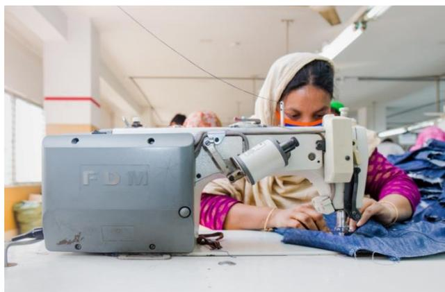
Workers using sewing machine equipped with servo motor at Bottom Gallery Pvt Ltd, Dhaka
